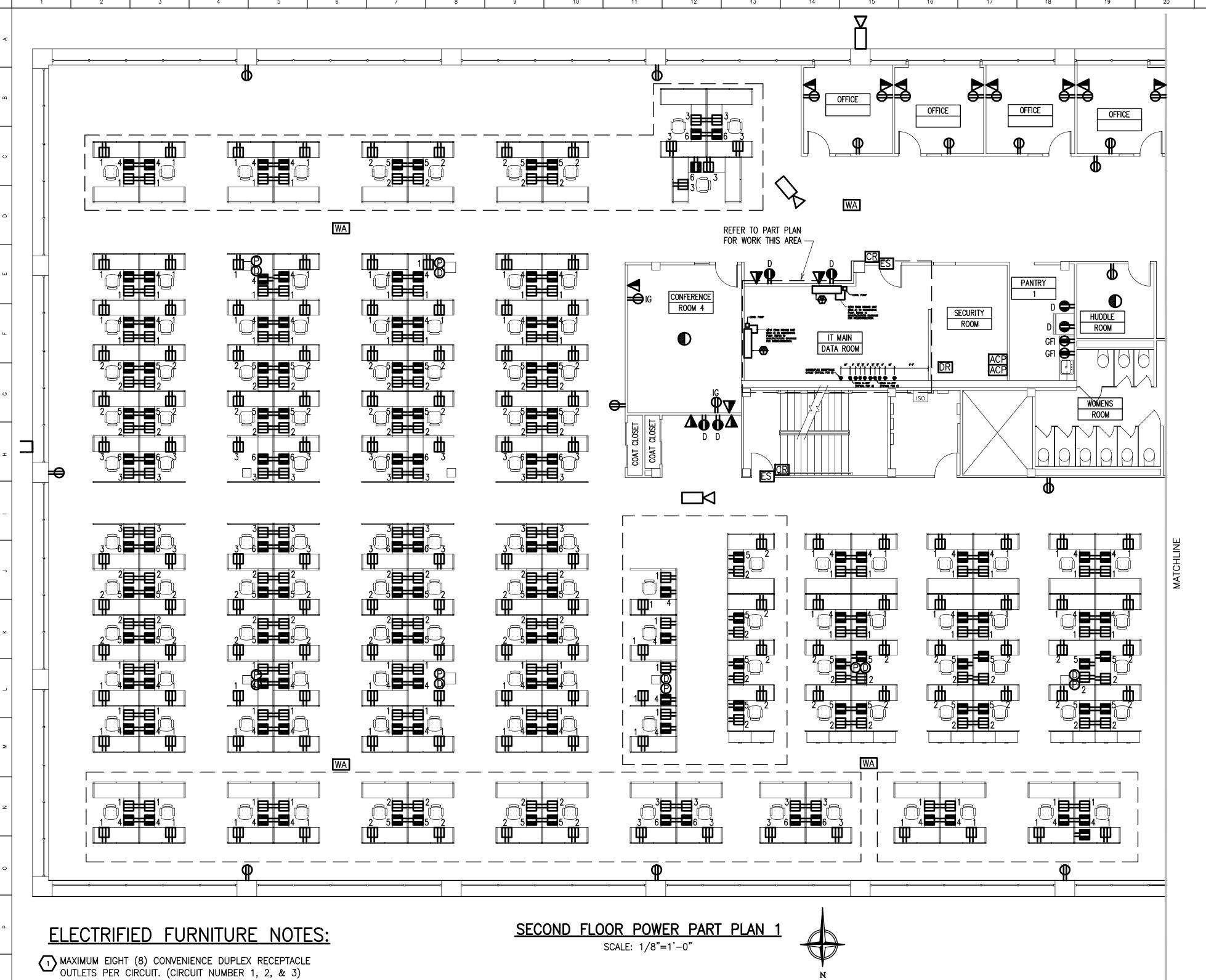
MAXIMUM FOUR (4) DUPLEX RECEPTACLE OUTLETS PER CIRCUIT FOR COMPUTERS. (CIRCUIT NUMBER 4, 5, & 6)
