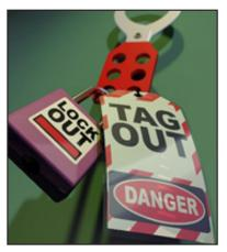
A designated employee is responsible for turning off and disconnecting the machinery or equipment from its energy sources prior to performing service or maintenance. This trained, authorized employee locks and/or tags the energy-isolating device and takes any additional steps needed to prevent the release of hazardous energy.
