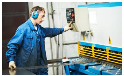
No New Hazards: Guards defeat their own purpose if they create hazards of their own. The edges of guards, for example, should be rolled or bolted to eliminate sharp edges.
